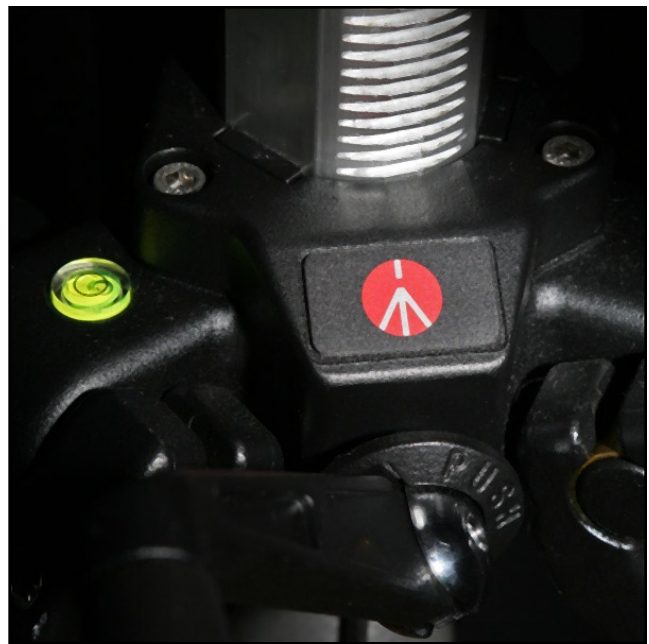
A close up image of a geared center column. Note the addition of a circular level to indicate how level the tripod's legs are positioned.
